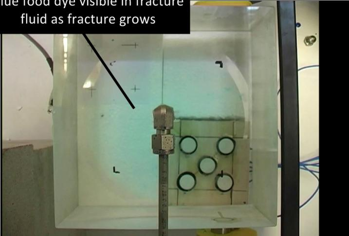
Glass sample containing hydraulic fracture
