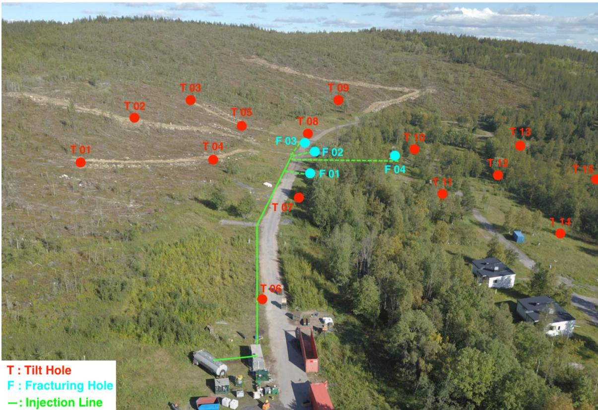
CSIRO's Preconditioning Site and Tilt Monitoring Array
