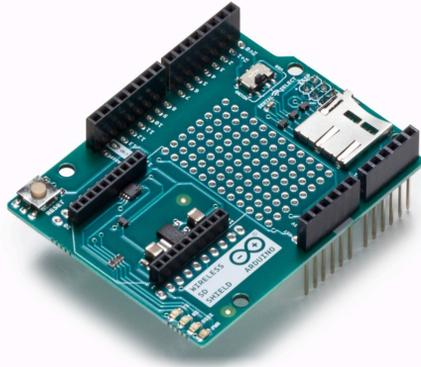
**Arduino Wireless SD Shield**
