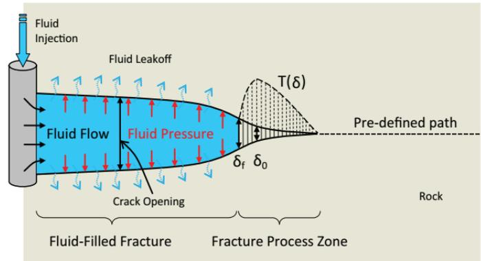
Figure 1. Cohesive zone hydraulic fracture model (After Chen (2012)).
