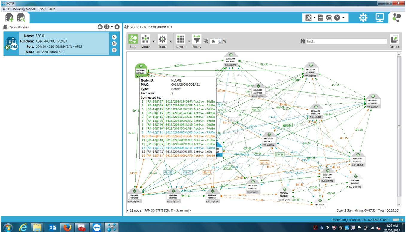
XCTU software for monitoring the connection quality of XBee radio transceivers.
