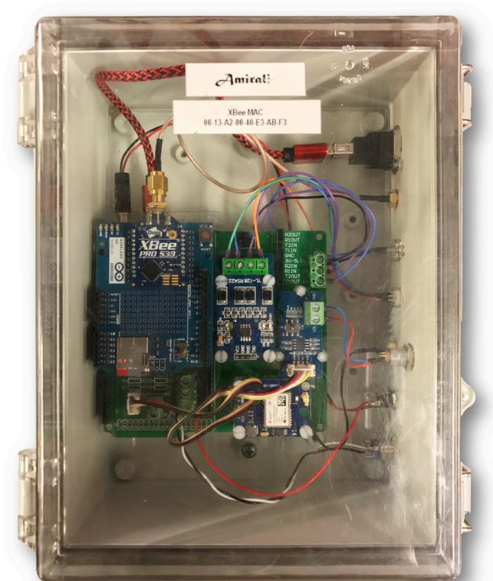
Radio Module Box – Hardware cost: **250 AUD** per node
