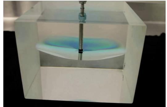
Labscale hydraulic fracture experiments in Glass
